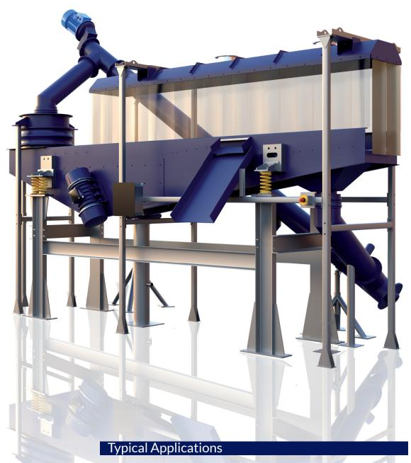
Separation of light metals (aluminum and magnesium) from heavy metals from fines and mid sizes zorba (3/16" up to 1 1/2")
